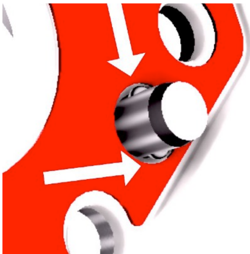
Fig.4: Check if ball locking pushpin's balls are visible before use
